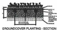
GROUND COVER PLANTING - SECTION
