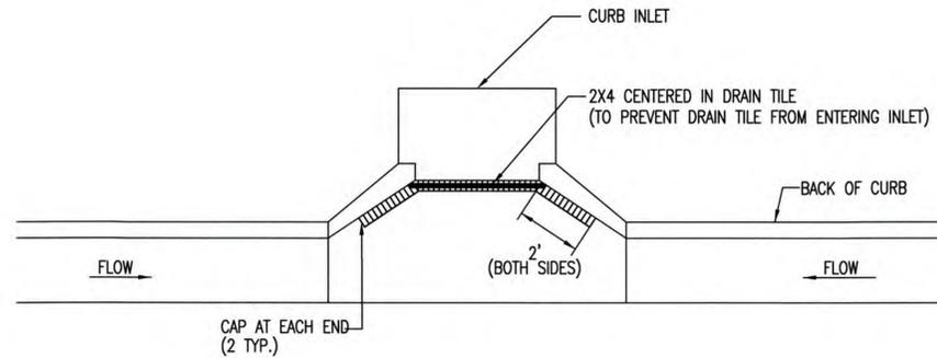
NOTE: PLACE 4" PERFORATED PVC PIPE, FILLED WITH 1/2"-1" DIA. GRAVEL, IN FRONT OF CURB INLET AS SHOWN.
