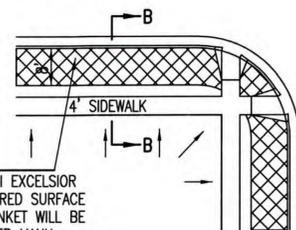
INSTALL 8" WIDE CURLEX I OR II EXCELSIOR BLANKET, OR EQUAL, ON PREPARED SURFACE BACK OF CURB. EDGE OF BLANKET WILL BE AT BACK OF CURB. INSTALL PER MANUFACTURERS RECOMMENDATION, INCLUDING STAPLES. (SEE DETAIL)
