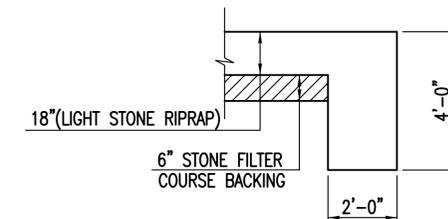
**TYPICAL SECTION THRU TOEWALL**
