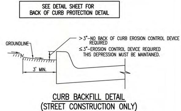
THIS IS A TEMPORARY MEASURE ONLY, WHEN APPROVED BY THE PROJECT ENGINEER. THE DIRT GRADE BEHIND THE CURB SHALL BE BROUGHT TO THE TOP OF CURB, WITH TEMPORARY EROSION CONTROL MAT OR PERMANENT VEGETATION PLACED, PRIOR TO THE COMPLETION OF ALL PROJECTS.
