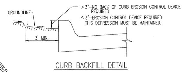
THIS IS A TEMPORARY MEASURE ONLY, WHEN APPROVED BY THE PROJECT ENGINEER. THE DIRT GRADE BEHIND THE CURB SHALL BE BROUGHT TO THE TOP OF CURB, WITH TEMPORARY EROSION CONTROL MAT OR PERMANENT VEGETATION PLACED, PRIOR TO THE COMPLETION OF ALL PROJECTS.
