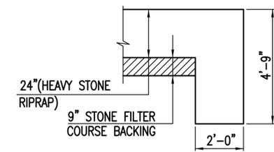
**TYPICAL SECTION THRU TOEWALL**
