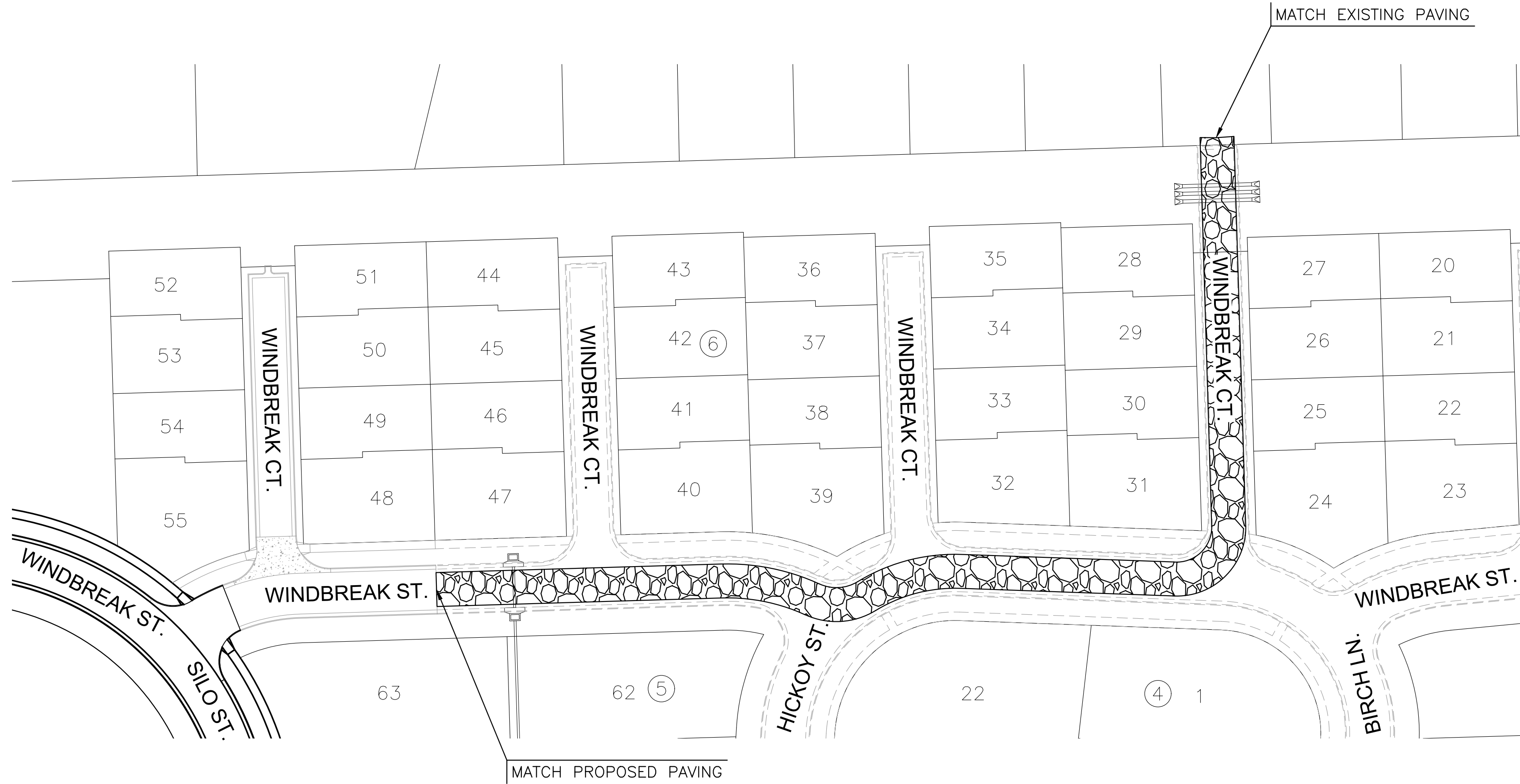
6" GRAVEL ACCESS ROAD SCALE: NTS
