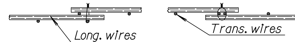
DETAIL OF LAP FOR WELDED WIRE REINFORCEMENT
