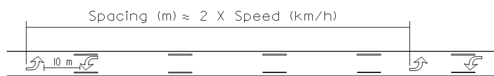
TWO-WAY LEFT TURN ARROW SPACING DETAIL
