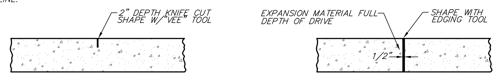
CONTRACTION JOINT (C.J.) OR LONGITUDINAL JOINT (L.J.) NO SAWN JOINTS WILL BE ALLOWED
