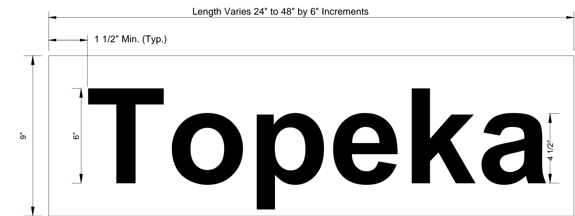
DETAIL A 9" STANDARD Length Varies 24" to 48" by 6" Increments
