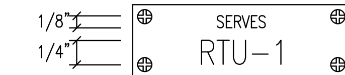
SWITCHBOARD/DISTRIBUTION PANEL/MOTOR CONTROL CENTER BREAKER/SWITCH
