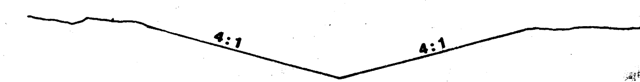
TYPICAL SWALE SECTION NTS
