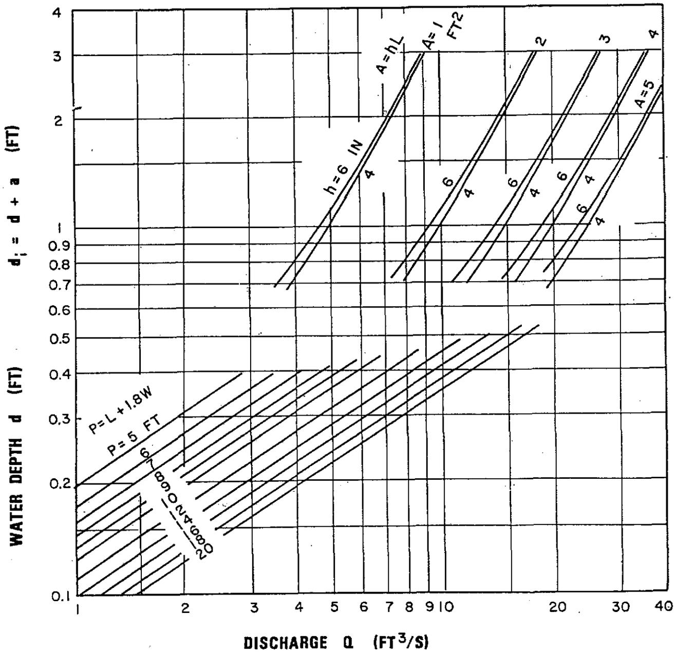
CHART 12. Depressed curb-opening inlet capacity in sump locations.
