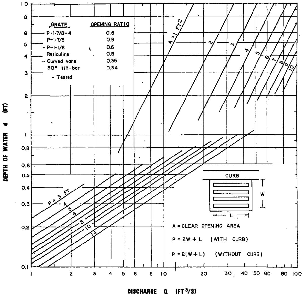
**CHART 11. Grate inlet capacity in sump conditions.**
