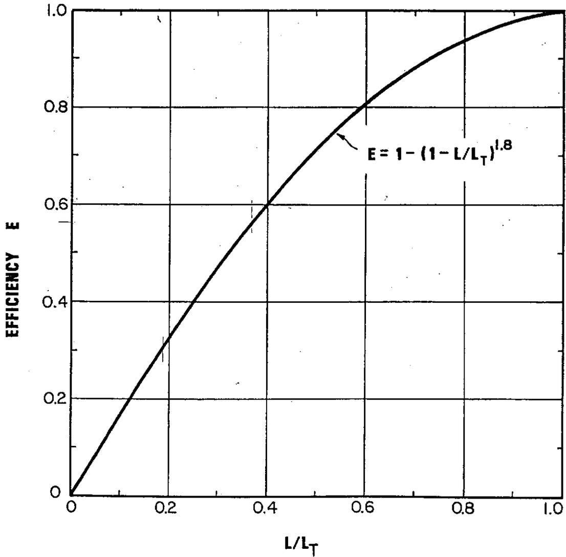
**CHART 10. Curb-opening and slotted drain inlet interception efficiency.**
