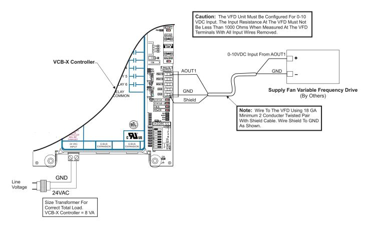
Figure 19: Supply Fan VFD Wiring
