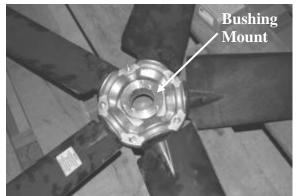
Figure 39 - Fan with the HUB on the Top and RET on the Bottom
