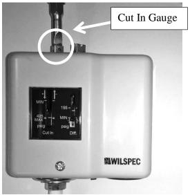
To lower the pressure set point for the **CUT IN** gauge, turn the adjustable screw clockwise.
