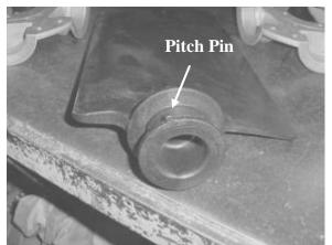
Figure 46 - Pitch Pin Location
