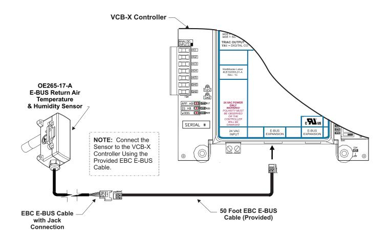
Figure 15: OE265-17-A – E-BUS Return Air Temperature & Humidity Sensor Wiring
