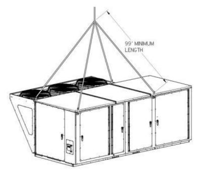
Figure 11 - Lifting Details of a 6-25 and 30 ton Energy Recovery Wheel or Power Return Unit
