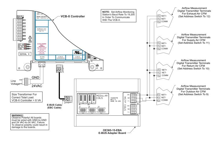
Figure 37: EBTRON<sup>®</sup> GTC116 Series, GreenTrol<sup>™</sup> GA-200-N Series, and Paragon MicroTrans<sup>EQ</sup> Series Air Flow Measurement Digital Transmitter Wiring
