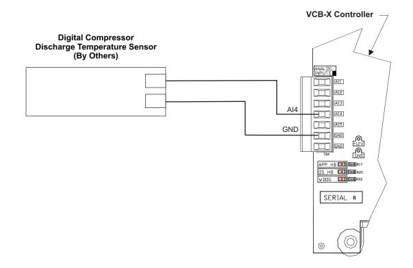
Figure 17: Digital Compressor Discharge Temperature Sensor Wiring
