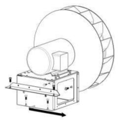
Figure 54 - Bolts which Connect Motor Mount to Blower Fan
