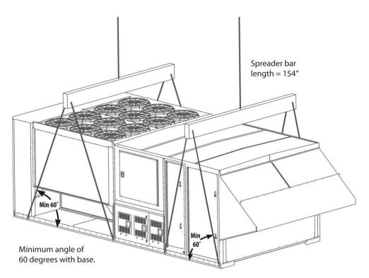
Figure 13 - Lifting Details of a 55, 65 and 75-140 ton Unit
