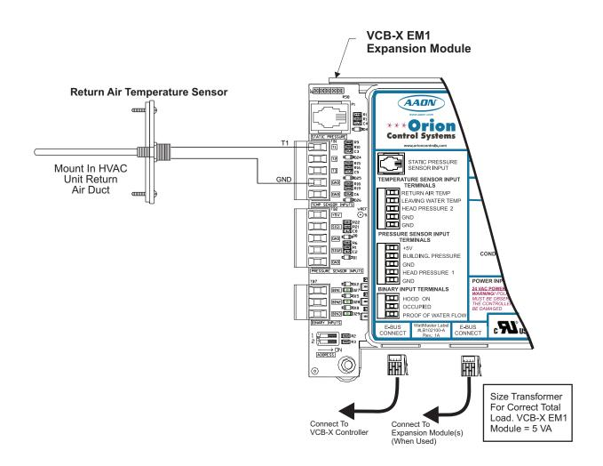
Figure 25: OE231 Return Air Temperature Sensor Wiring Diagram
