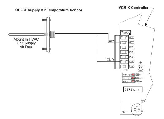
Figure 12: OE231 – Supply Air Temperature Sensor Wiring
