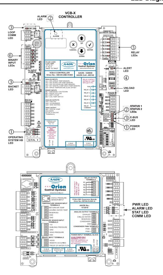
Figure 42: VCB-X Controller & VCB-X EM1 Expansion Module LED Locations
