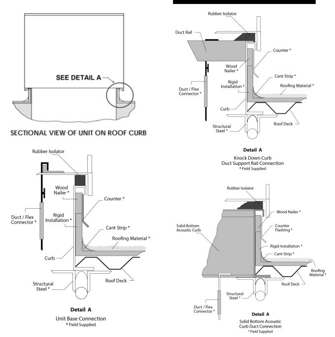
Figure 14 - Duct Connection
