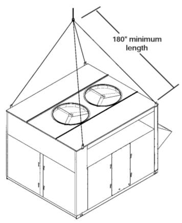
Figure 12 - Lifting Details of a 26, 31-50, 60 and 70 ton Unit
