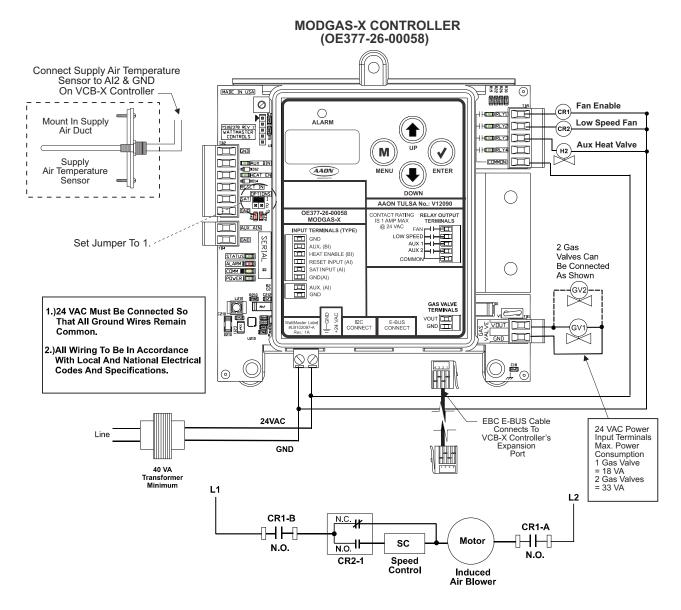
Figure 39: MODGAS-X Controller to VCB-X Controller Wiring Diagram
