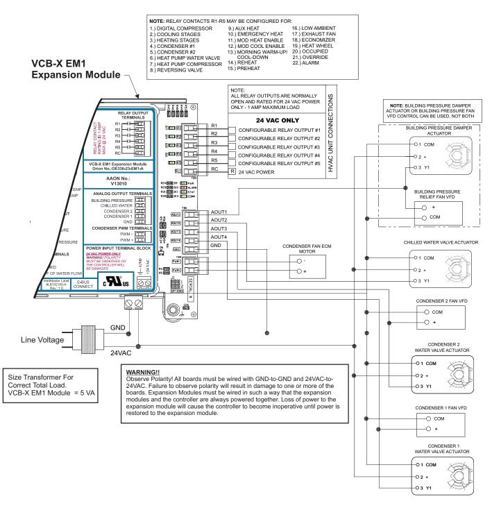
Figure 23: VCB-X EM1 Expansion Module Output Wiring Diagram
