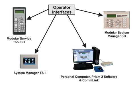
Figure 43: Available Operator Interfaces
