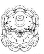
Top half is the HUB. Bottom half is the RET or retainer ring.
