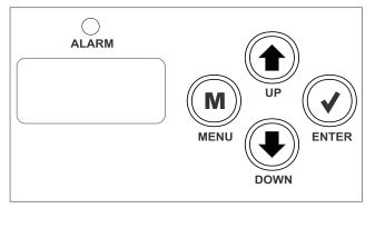
Figure 47: LCD Display and Navigation Keys
