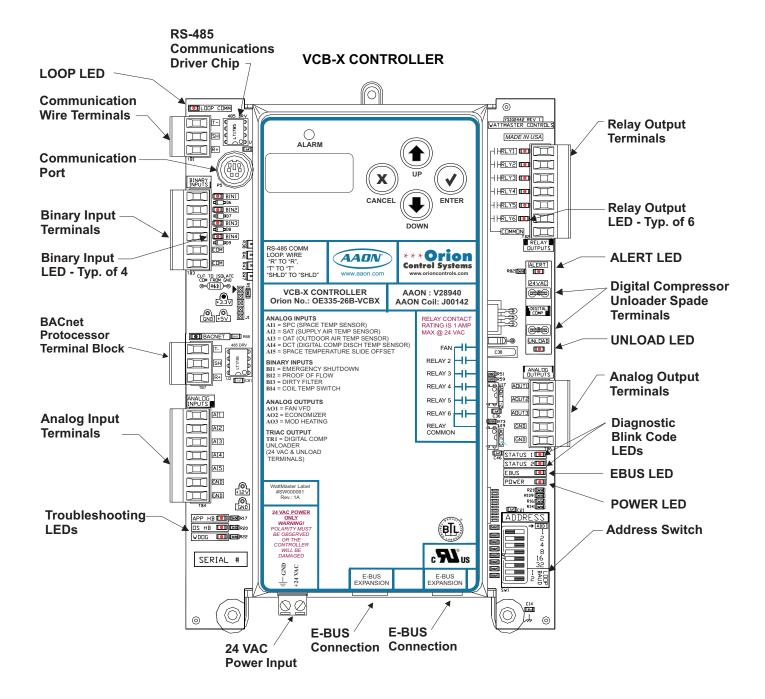
Figure 5: VCB-X Controller w/Enclosure Components
