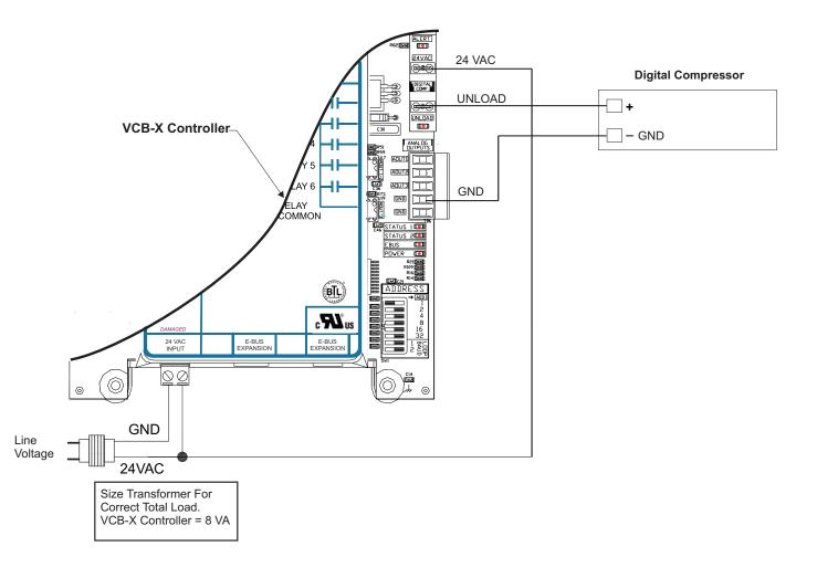
Figure 18: Digital Compressor Unloader Wiring
