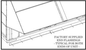
Figure 25 - Factory Supplied End Flashings
