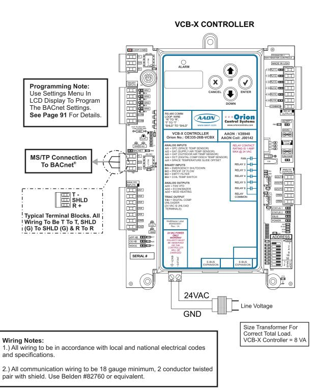
Figure 48: VCB-X BACnet Connection to MS/TP Network
