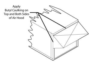
Figure 24 - 26 and 31-140 ton Open Rain Hood
