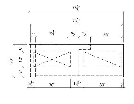
RN-B, Std 14 Gauge Galvanized Steel 1.5" Insulation on Walls 1" Insulation on Floor Turning Vanes in Supply Section Pad Mount
