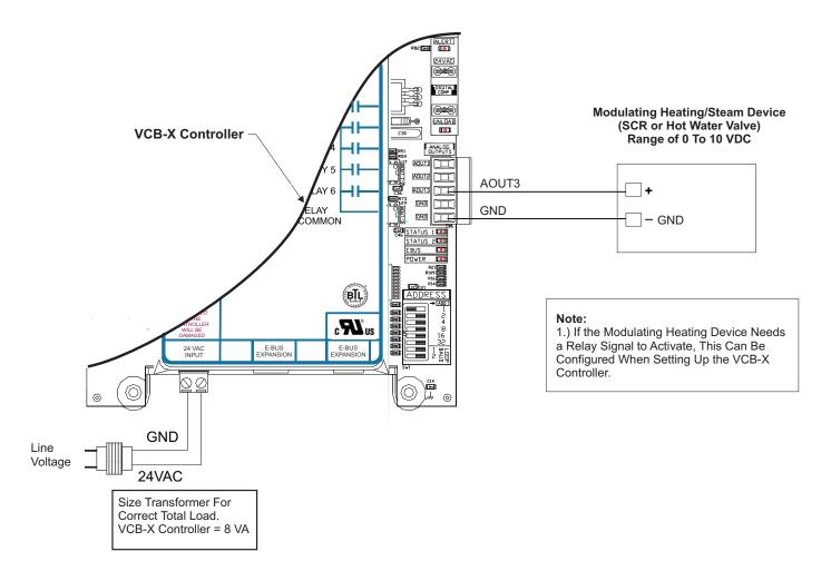
Figure 21: Modulating Heating Device Wiring
