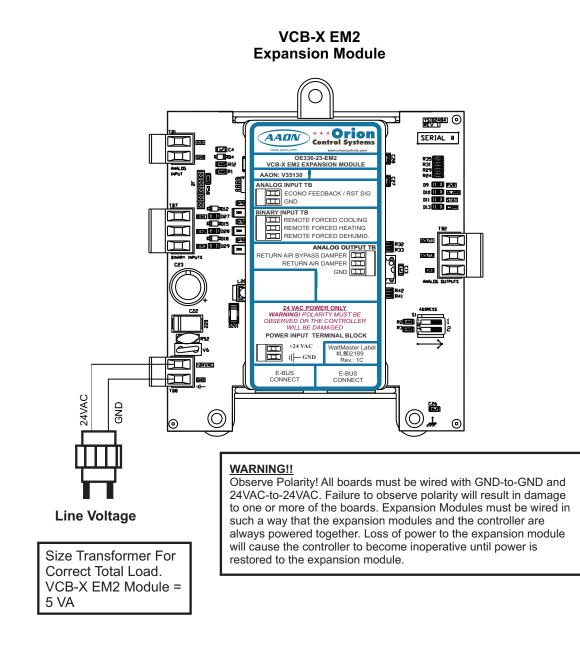
Figure 33: VCB-X EM2 Expansion Module
