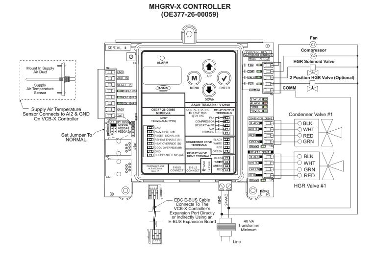
Figure 38: MHGRV-X Controller to VCB-X Controller Wiring
