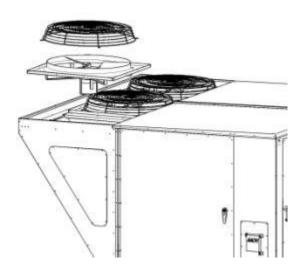
Figure 51 - Removal of a Condenser Fan Assembly
