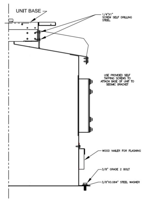
Figure 15 - Solid Bottom Seismic Curb with Filters
