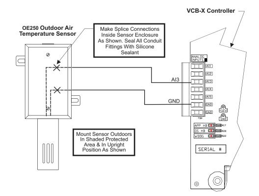
Figure 13: OE250 – Outdoor Air Temperature Sensor Wiring
