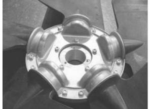
Figure 44 - Back of the Fan Step 4: Remove the fan blades and replace the pitch pins
