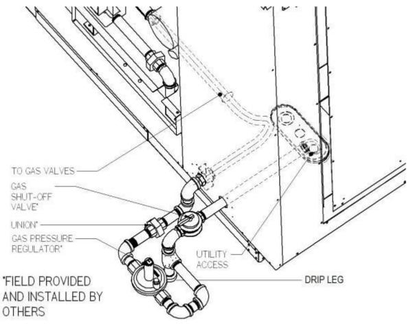
Figure 31 - Example 6-50, 60 & 70 ton through the Base Gas Piping
