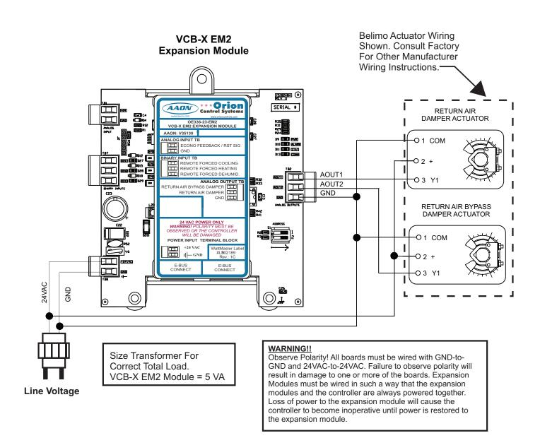
Figure 35: Return Air Bypass Wiring
