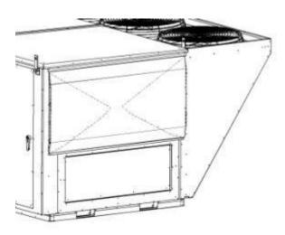
Figure 22 - 6-25 and 30 ton Closed Rain Hood
