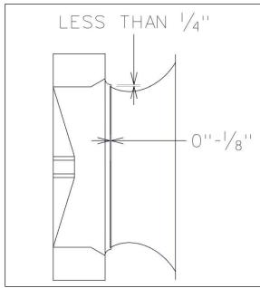
Figure 38 - Plenum Fan Gap Tolerances
