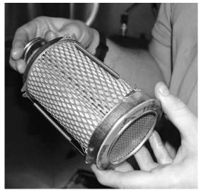
Figure 48 - RPE-48-BD filter element
