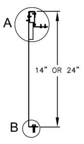
Figure 16 - Seismic Solid Bottom Curb without Filters Cross Section
