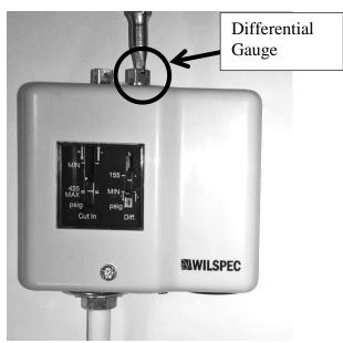
To raise the pressure set point for the **DIFFERENTIAL** Gauge, turn the adjustable screw clockwise.
