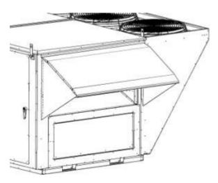
Figure 23 - 6-25 and 30 ton Open Rain Hood
