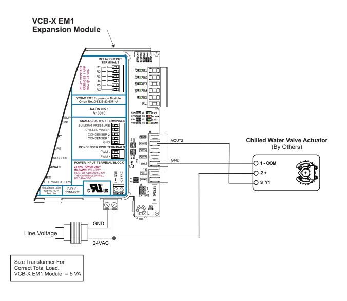
Figure 31: Chilled Water Valve Actuator Wiring Diagram
