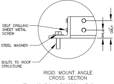
Figure 19 - Seismic Rigid Mount Curb
