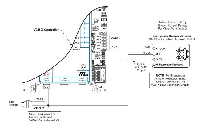
Figure 20: Economizer Damper Actuator Wiring
