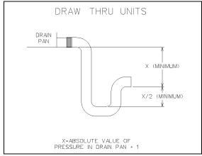
Figure 33 - Draw-Through Drain Trap
