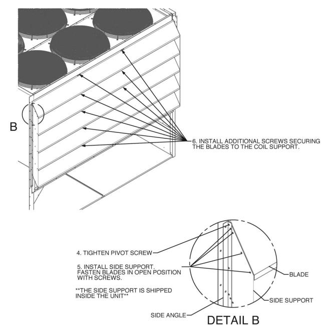
Figure 21 - 90-140 ton Condenser Coil Guard Installation Instructions 2
