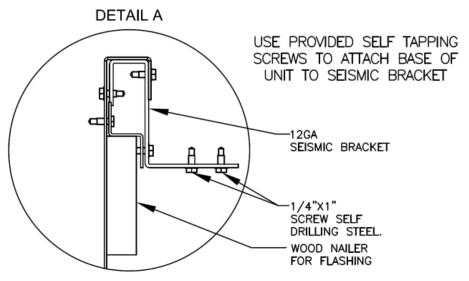
Figure 17 - Seismic Solid Bottom Curb without Filters Detail A
