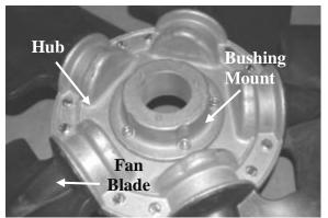
Figure 43- Assembled Fan
