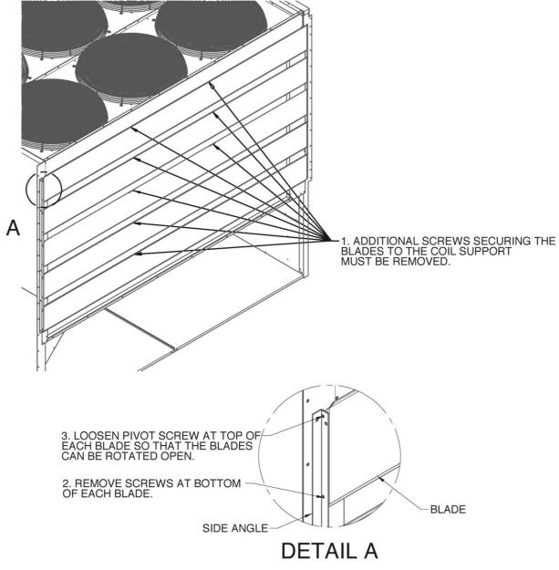
Figure 20 - 90-140 ton Condenser Coil Guard Installation Instructions 1
