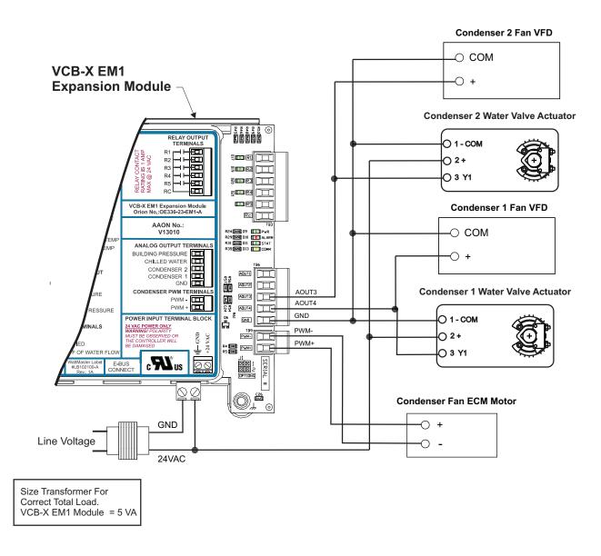
Figure 32: Condenser Fan ECM Motor and (2) Condenser Fans VFD or (2) Condenser Water Valves Actuator Wiring Diagram
