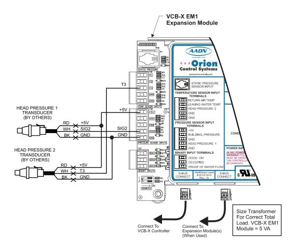
Figure 29: Head Pressure Transducers Wiring Diagram
