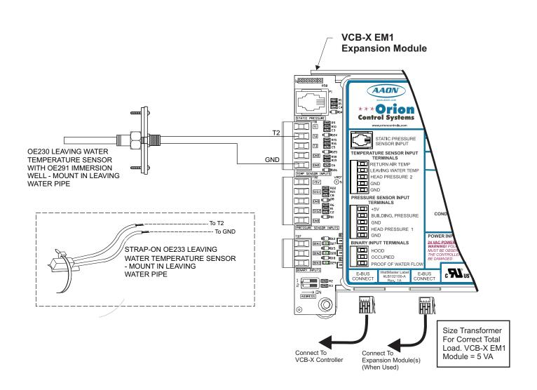
Figure 26: OE230 and OE233 Leaving Water Temperature Sensor Wiring Diagram
