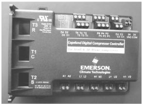
Figure 55 - Variable Capacity Compressor Controller
