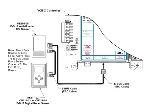
Figure 9: OE256-05 – Wall Mounted E-BUS CO<sub>2</sub> Sensor Wiring
