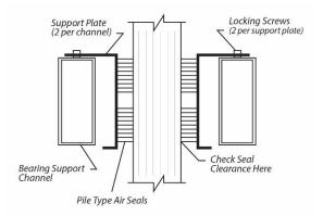
Cross Section of Air Seal Structure
