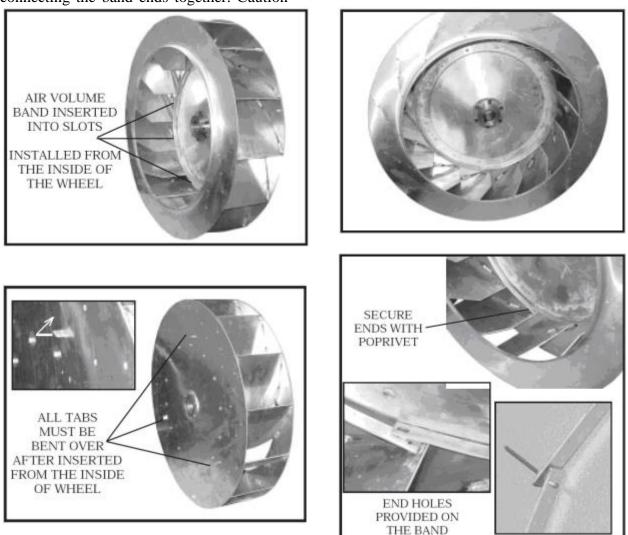
Figure 37 - Supply Fan Banding
