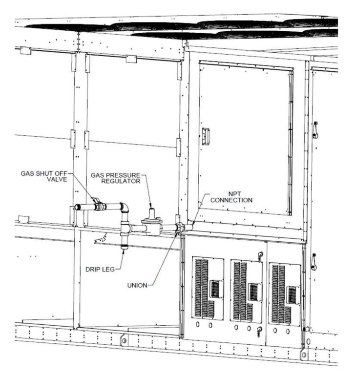
Figure 32 - Example 55, 65 and 75-140 ton for across the Roof Gas Piping Note: There will be two gas connections, one on each side of the unit
