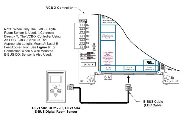
Figure 8: OE217-02, OE217-03, OE217-04 - E-BUS Digital Room Sensor Wiring
