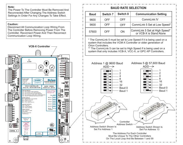
Figure 40: VCB-X Controller Address Switch and Baud Rate Setting
