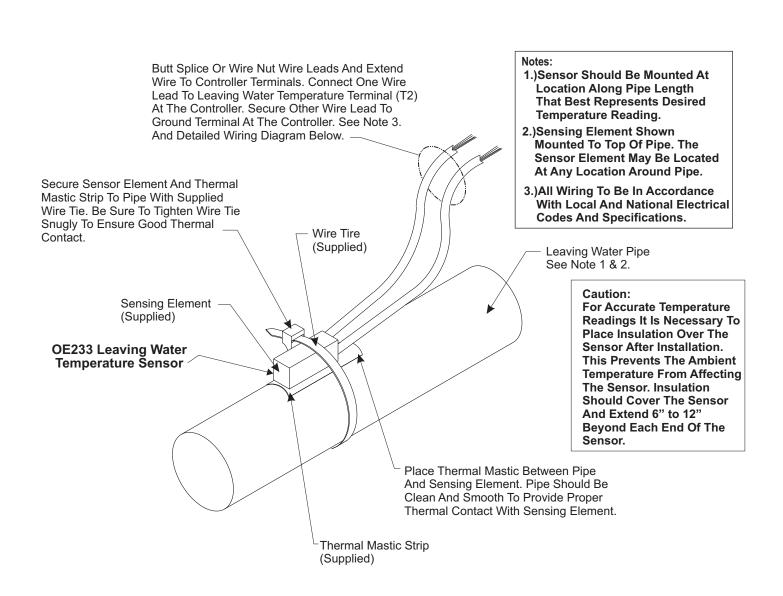
Figure 27: OE233 Strap-On Leaving Water Temperature Sensor Installation
