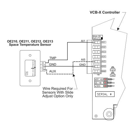
Figure 11: OE210, OE211, OE212, OE213 – Space Temperature Sensor Wiring and Slide Adjust
