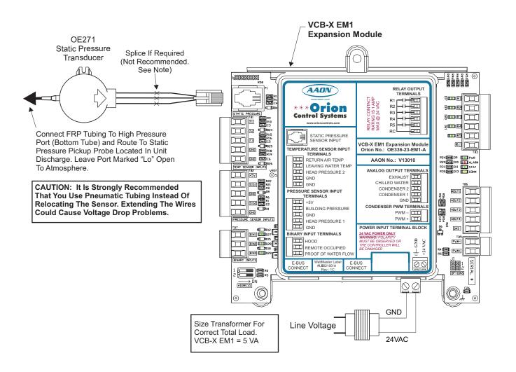
Figure 24: OE271 Static Pressure Transducer Wiring Diagram
