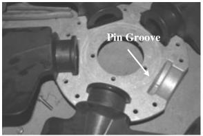
Figure 45 - Pin Groove Location
