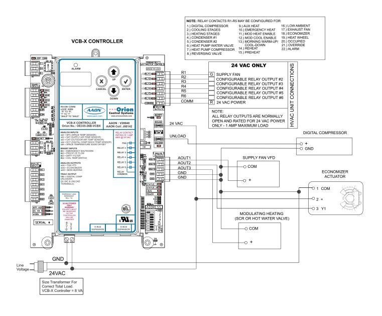
Figure 7: VCB-X Controller Output Wiring
