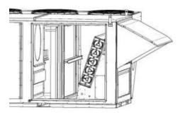
Figure 52 - Evaporator Coil Access
