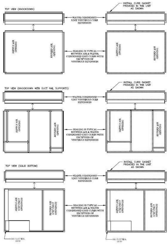
Figure 6 - RN Series 9 and 11-15 ton Unit Isolator Locations
