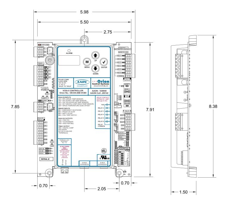
Figure 1: VCB-X Controller Dimensions
