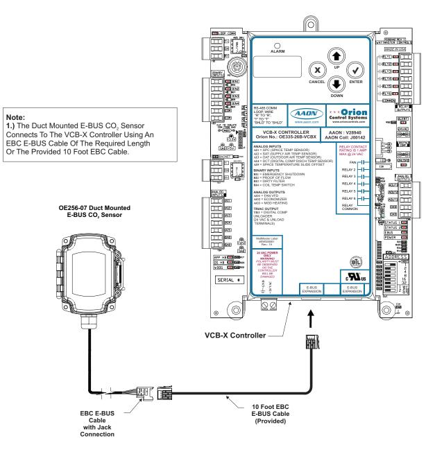
Figure 10: OE256-07 - Duct Mounted E-BUS CO, Sensor Wiring
