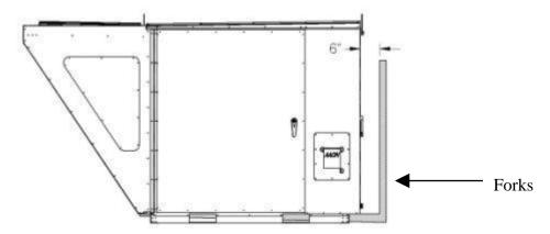
Figure 9 - Forklifting an RN Series A, B and C Cabinet, 6-25 and 30 tons
