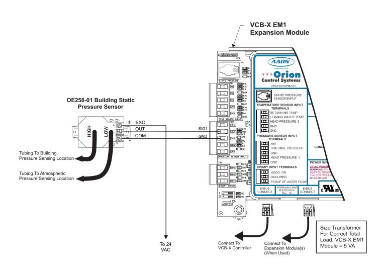
Figure 28: OE258-01 Building Static Pressure Sensor Wiring Diagram
