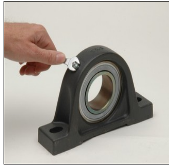
Remove grease nipple from bearing with wrench
