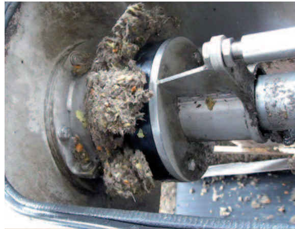
Discharge of the separated pressed material
