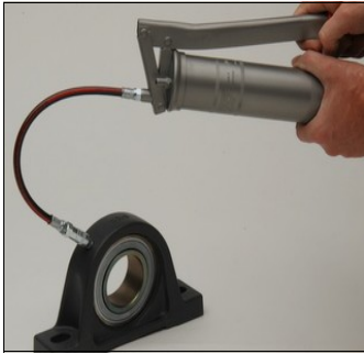
Pre-grease bearing with lever grease gun
