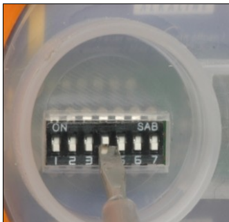
Set DIP-switches to select grease discharge setting (see table)
