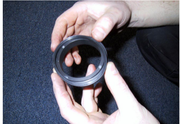
Picture 5.28 Installing Smaller Quad Ring on The Carbon
