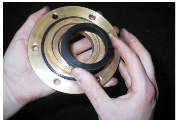
Picture 5.29 Installing Carbon into Seal Housing
