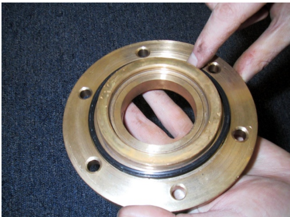
Picture 5.27 Installing Larger Quad Ring into The Seal Housing
