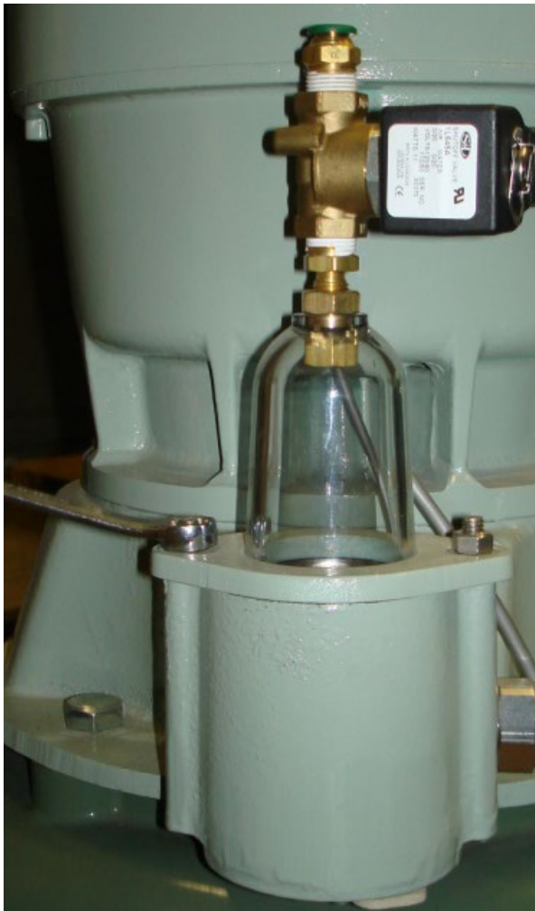
Picture 5.41 Removing the Retaining Ring Fasteners
