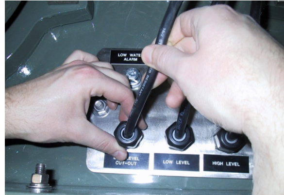
Picture 3.2 Adjusting Cords Through Cord Grip
