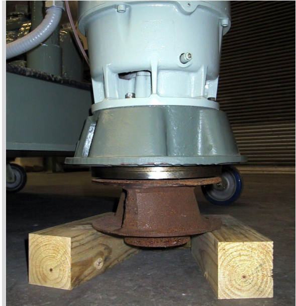
Picture 5.21 Impeller Resting on Two (2) 4" x 4" Boards
