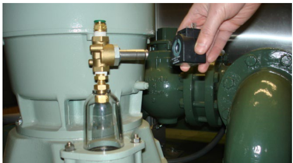
Picture 5.47 Removing Solenoid Valve Coil
