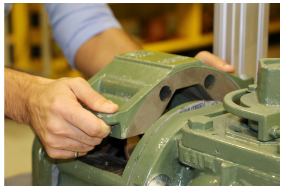
Picture 5.3.B Removing Valve Top
