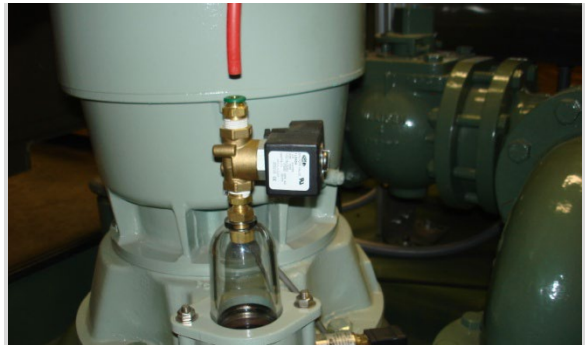
Picture 5.16 Removing the Vacuum Tubing
