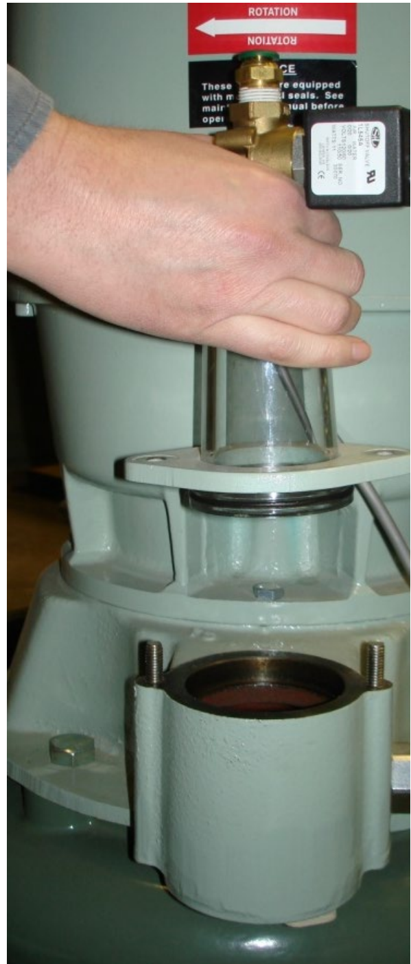
Picture 5.42 Removing the Retaining Ring
