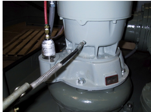
Picture 5.1 Lubricating Motor
