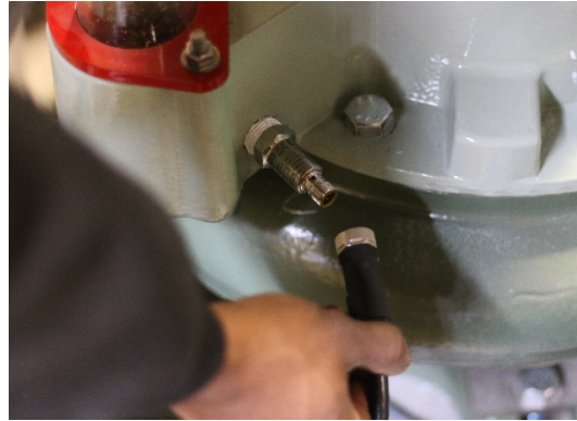
Picture 5.15 Removing the WaveStart™ Cable
