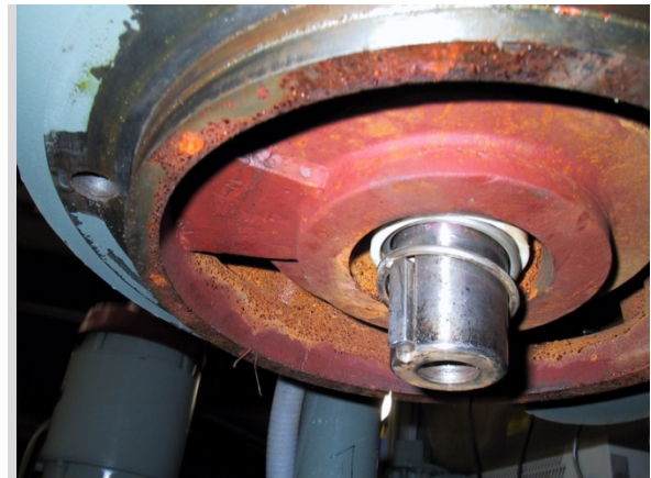
Picture 5.33 Motor Shaft with Key, Spring and Ceramic Installed
