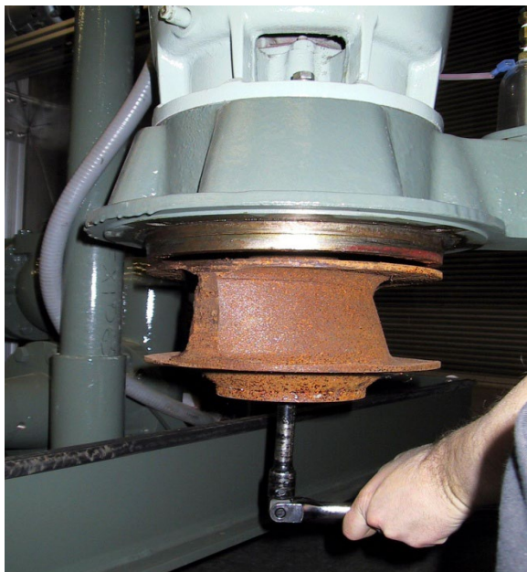
Picture 5.20 Loosening the impeller bolt.
