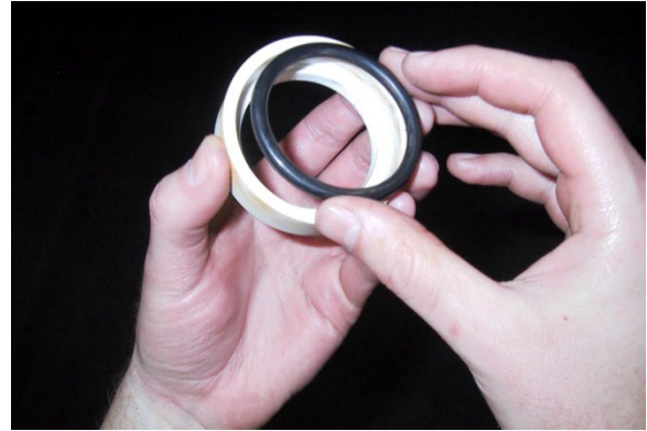
Picture 5.32 Installing “O”-Ring Inside the Ceramic
