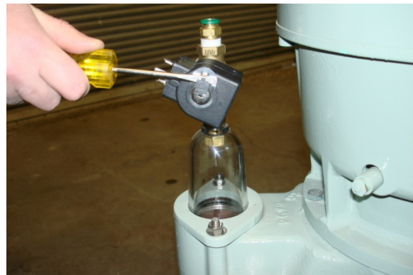
Picture 5.46 Removing Solenoid Valve Retaining Clip
