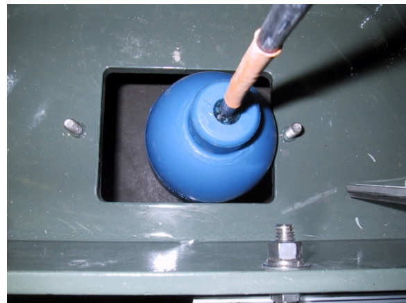
Picture 3.3 Lowering Float Through Baseplate.
