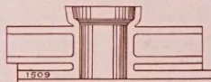
Cut No. 1509—T-Branch Segment Sewer Block Branches or Junctions, Segment Block Fittings
