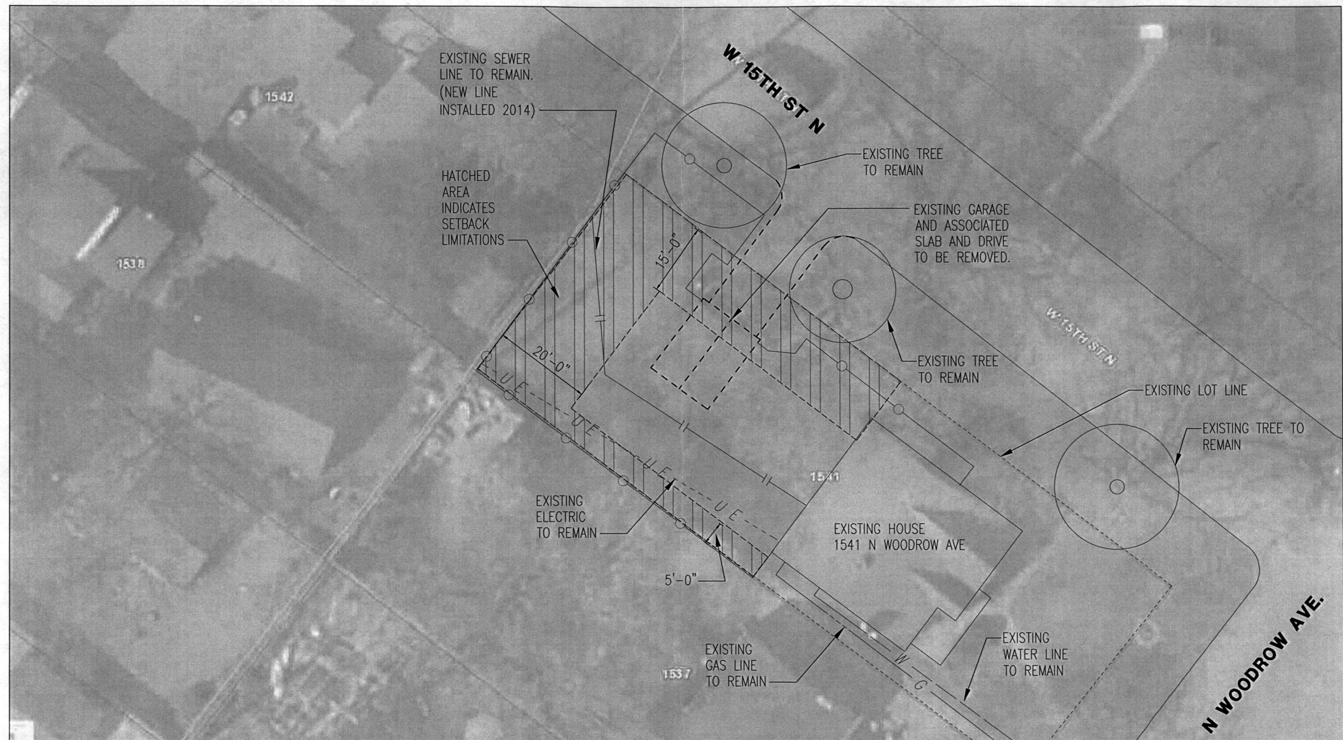
A EXISTING SITE PLAN 0' 10' 20' 30' 50' SCALE: 1" = 20'-0"
