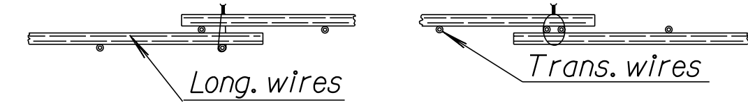
DETAIL OF LAP FOR WELDED WIRE REINFORCEMENT
