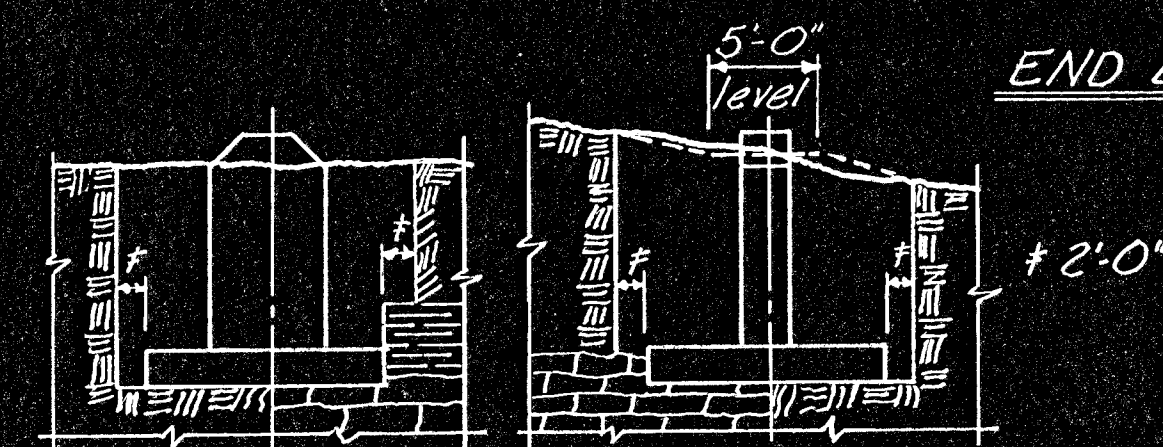
Side Elev. End Elev. TYPICAL EXCAVATION DETAILS
