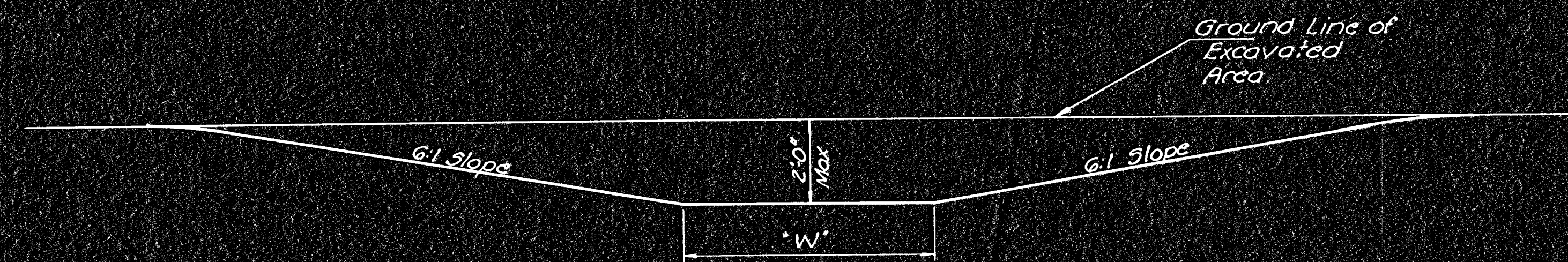
TYPICAL SECTION OF OUTLET DITCH
