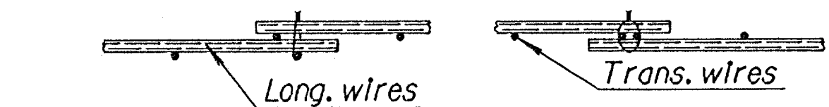
DETAIL OF LAP FOR WIRE MESH The lap shall extend beyond the first transverse or bag wire of each sheet. The sheet shall be wired securely at the edges and at intervals not to exceed 750 mm for the full width of the sheet. Approximate weight of wire mesh = 2.8 kg per m 2 . Other methods for fastening the sheets of wire mesh at the laps may be used with the approval of the Engineer.
