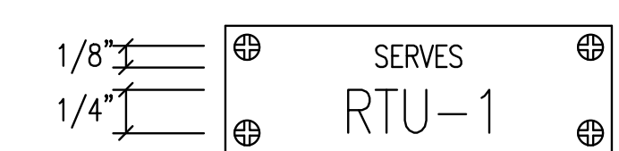
SWITCHBOARD/DISTRIBUTION PANEL/MOTOR CONTROL CENTER BREAKER/SWITCH
