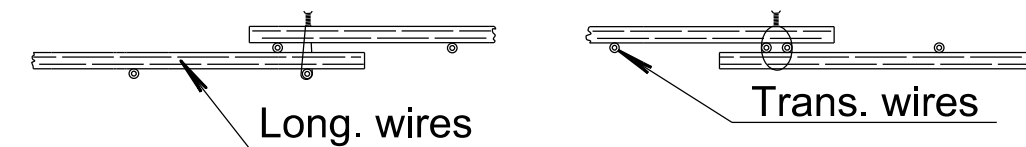
DETAIL OF LAP FOR WELDED WIRE REINFORCEMENT
