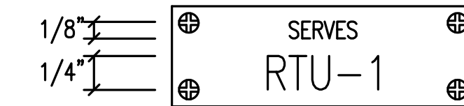
SWITCHBOARD/DISTRIBUTION PANEL/MOTOR CONTROL CENTER BREAKER/SWITCH
