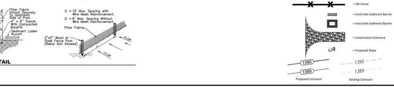
4 SILT FENCE DETAIL NOT TO SCALE
