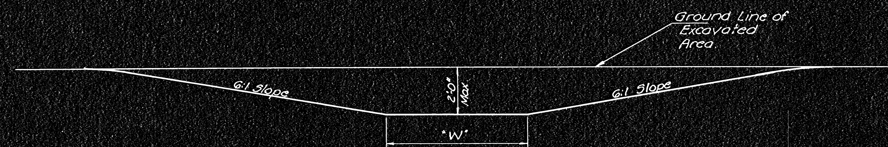
TYPICAL SECTION OF OUTLET DITCH
