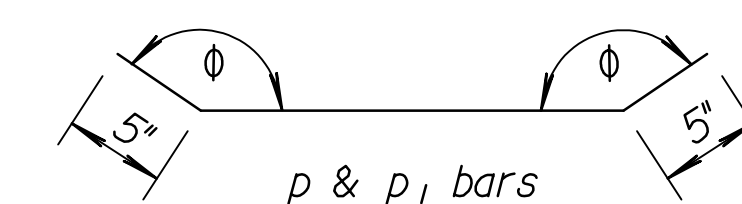
\phi Angle varies according to skew of RCB. Bars shall be field bent.
