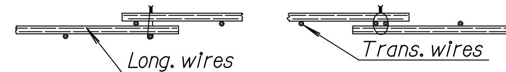
DETAIL OF LAP FOR WELDED WIRE REINFORCEMENT
