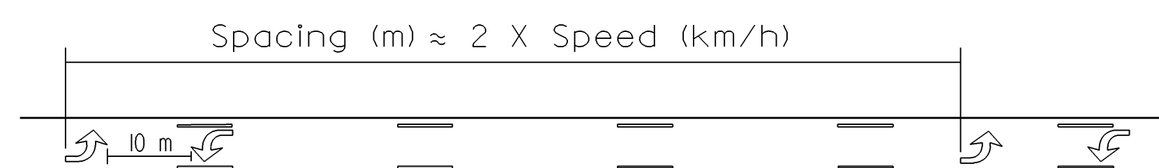
TWO-WAY LEFT TURN ARROW SPACING DETAIL
