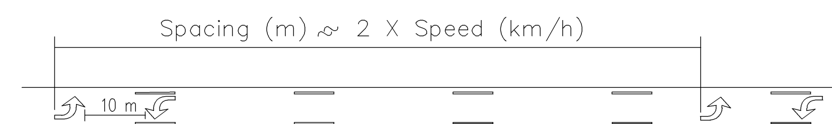
TWO-WAY LEFT TURN ARROW SPACING DETAIL
