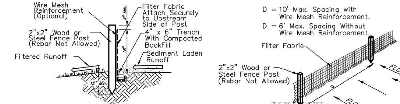
1 SILT FENCE DETAIL NOT TO SCALE
