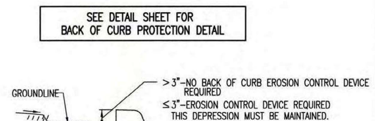
CURB BACKFILL DETAIL (STREET CONSTRUCTION ONLY)
