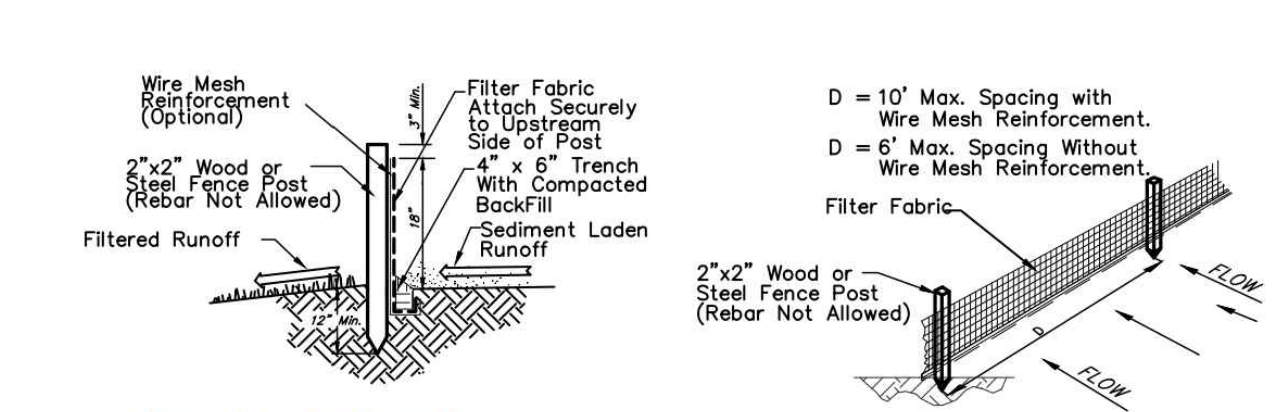
2 SILT FENCE DETAIL NOT TO SCALE
